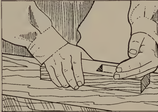
Figure 5.11. Correct way to hold the plane.
