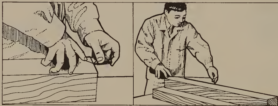
Figure 4.6. Marking a line with the sumitsubo .
