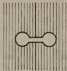
Are kata —Dumb-bell. Not used for architectural construction. [But used for cabinetry in the west.]
