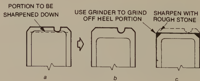
Figure 2.58. Grinding a damaged blade.
