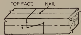
Arikaki tsugi — Oblique surfaced half-lap joint.
