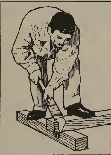
Figure 5.3. Correct position for crosscutting.
