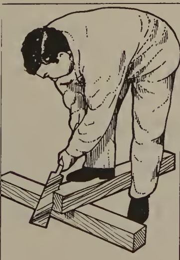
Figure 5.4. Correct position for rip cutting.
