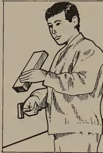
Figure 2.44. Setting the blade.
