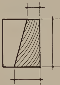
Figure 6.76. Pattern for cutting nageshi .
