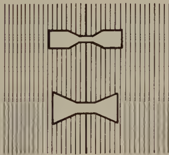
Kine kata —Bow-tie spline (2 types).
