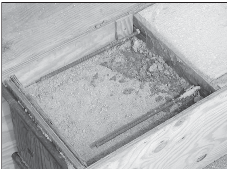
Figure 8. Laboratory test illustrating one method of pouring concrete bond beam in top of rammed earth forms, holding concrete back to allow for a rebar splice
