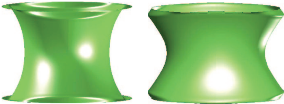
Figure 4.25 The deformed configuration viewed from two different angles. Compression lobes are visible where the loading is directed inward. Expansion lobes are visible where the loading is directed outward.
