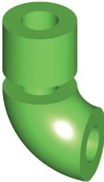
Figure 2.36 The pipe has two basic sections: a cylinder and an elbow. We must choose a knot vector that respects both of these distinct pieces, while allowing us to join them into one geometrical object.
