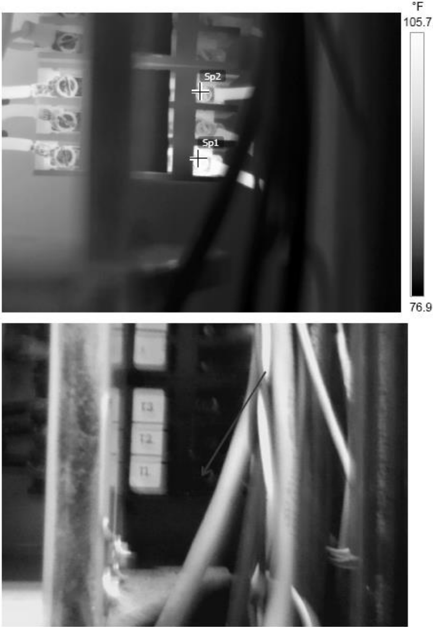
Figure 7.2-2. Motor Control Center (MCC) Thermal Scan of a Phenol Unit - Photo 2
