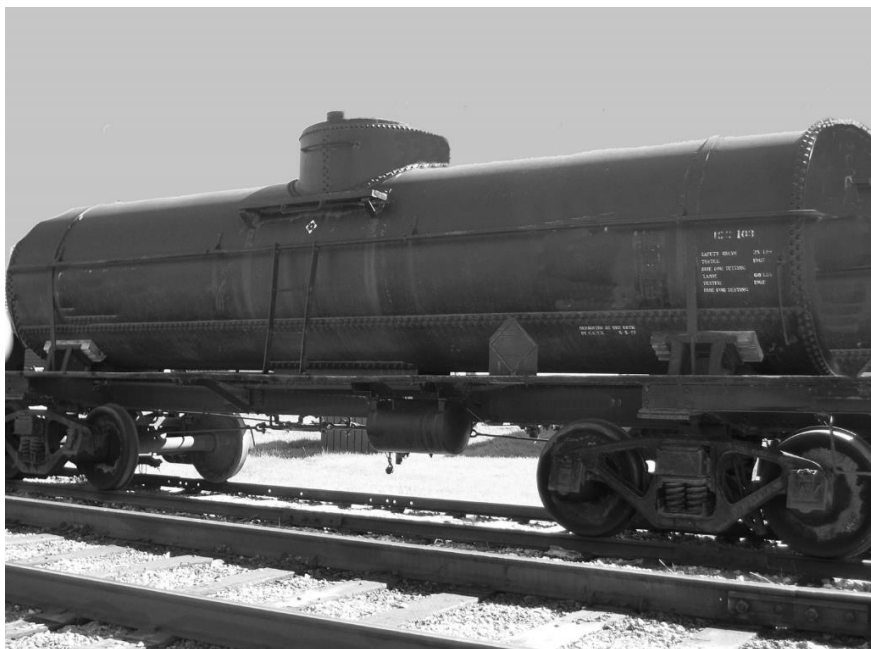
Figure 7.3-1. Picture of Vintage Tank Car Fastened with Rivets
