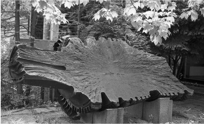
Figure 2.3-2. Catastrophic Failure of Electrical Generator Rotor
