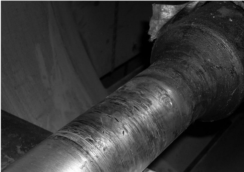
Figure 1.4-3. Image Showing Scoring on a Shaft
