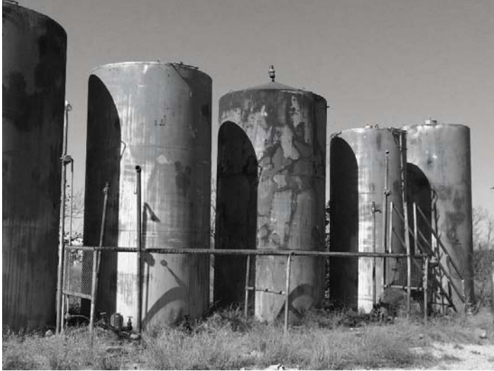
Figure 2.5-2. Image of Corroded Oil Recovery Vessels
