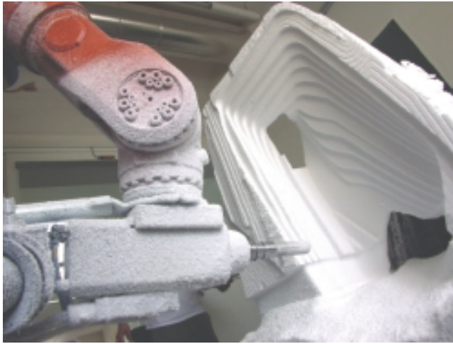
Figure 7.2 Kuka industrial robot milling a piece of the Genus 2 Lamp by SPAN. (Photo © SPAN 2008.)
