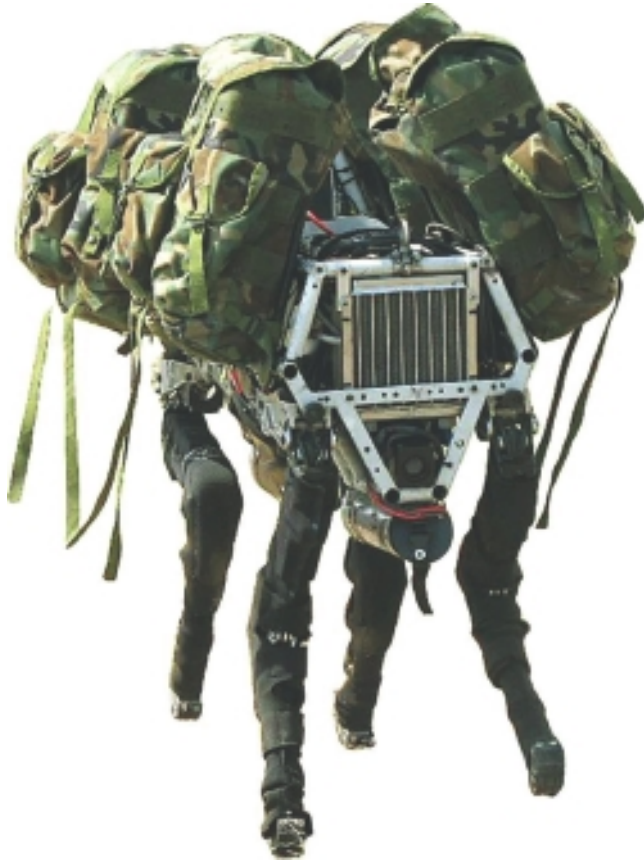
Figure 7.1 Big Dog rough-terrain robot by Boston Dynamics. (BigDog image courtesy of Boston Dynamics ©2009.)
