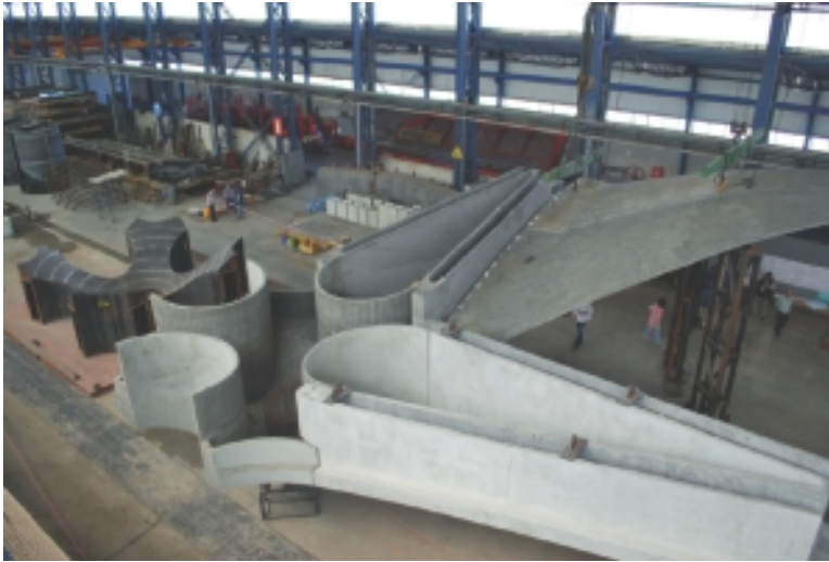
Figure 15.8 Queen Alia Airport, prefabricated concrete parts and formwork: Column head, beam and roof shell. (Image credit and copyright Foster + Partners.)
