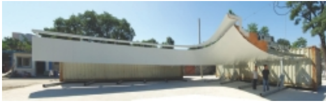
Figure 13.7 Façade mock-up: Sheet metal facade 1:1 test mock-up built in Beijing for SOHO Galaxy project, October 2009. (Reproduced by permission of Zaha Hadid Architects.)
