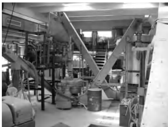
Fig. 5.25 Technical realization for direct contact drying of manure and sludge with zeolite, including zeolite regeneration. Zeolite transport from separator to regenerator to dryer is realized by two conveyor belts.
