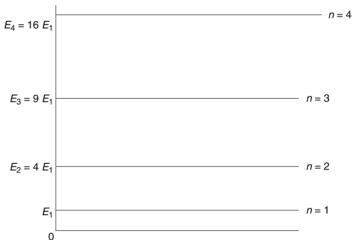
Figure 6.7 Energy-level diagram of particle in a one-dimensional box
