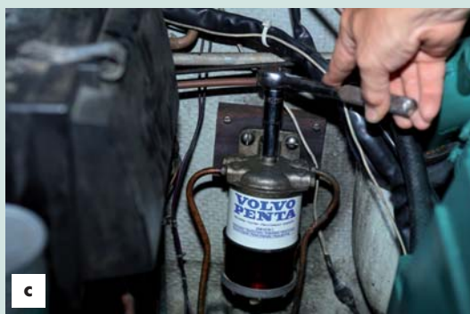
Fitting a new cartridge
