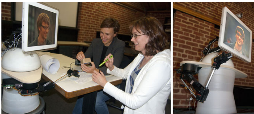
Fig. 1 An embodied communication avatar. The left panel shows the avatar in use during a distributed team working session. The right panel shows the avatar's screen, which carries the video feed of a remote participant, and its articulating neck, which is mounted to a stable base. These components represent a person's head, neck and upper torso, respectively. An expressive robotic arm, which the remote participant can control to point, wave, touch, and even tap against the table, is attached to one side
