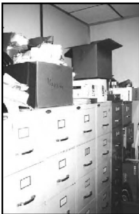
Figure 7-5. File cabinets with the hazard from the fall or shift of materials on top of them.
