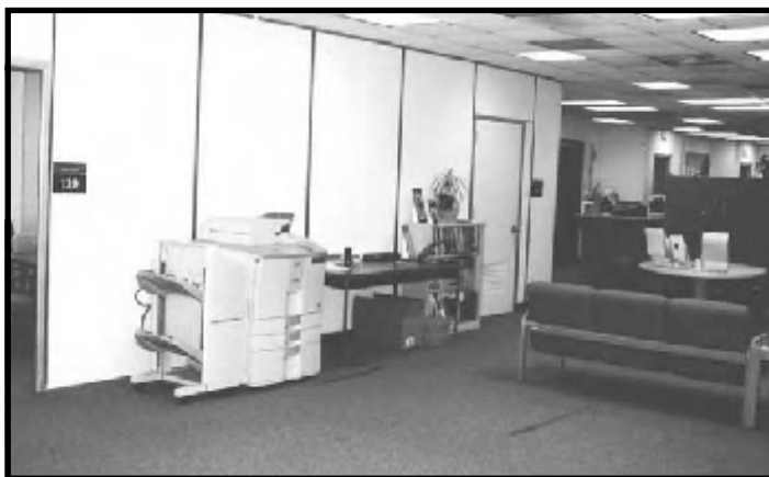
Figure 27-1. Common office area with unsecured carpet in main walking area.
