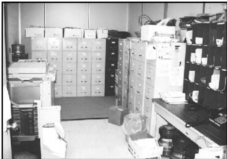
Figure 7-1. Any of these file cabinets could tilt onto a worker. Open file draws one at a time and close prior to opening another drawer.
