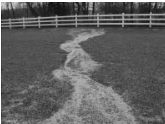
Figure 17.2. Rubber pieces can float to the top of a footing mixture after large rainfall events. The rubber will have to be mixed back into this stonedust mixture with surface conditioning equipment.
