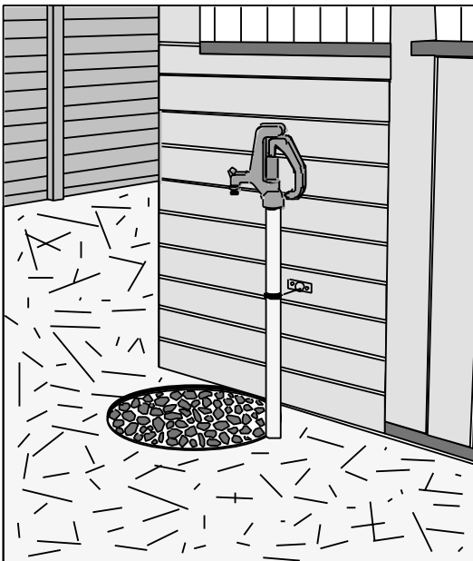
Figure 6.3. Design detail for freezing conditions, such as the self-draining water hydrant, will be needed in most horse stables located in cold climates.
