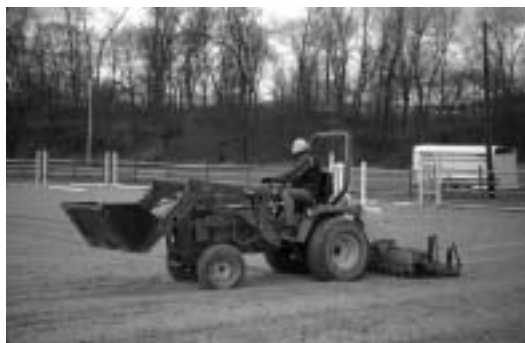
Figure 17.7. Equipment will be needed for frequent conditioning of the riding surface to redistribute footing for an even coverage of the base material and, in some cases, to loosen compacted surface materials.
