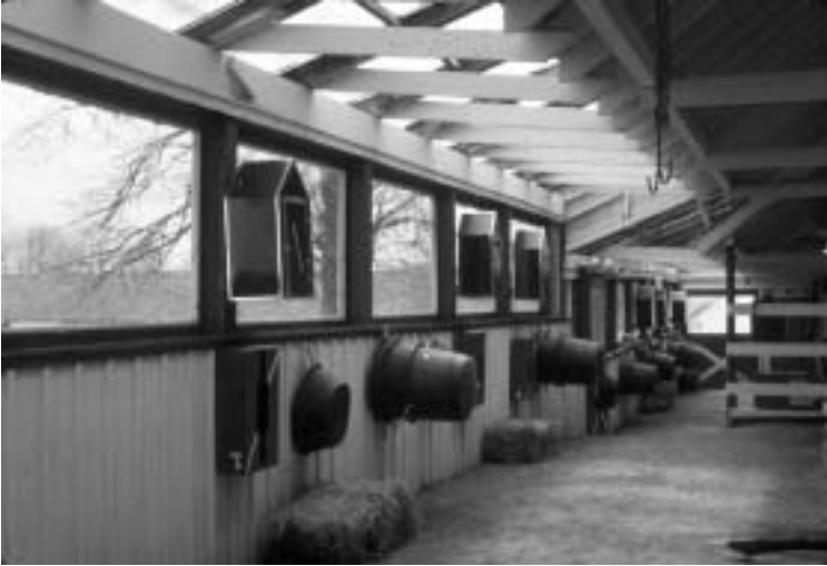
Figure 11.14. Conversion of this stable from open shed row design to an enclosed work aisle included provision for plenty of light for bright working conditions. Solar gain through roof plexiglass panels is welcome during cool weather but would be a liability on hot days.
