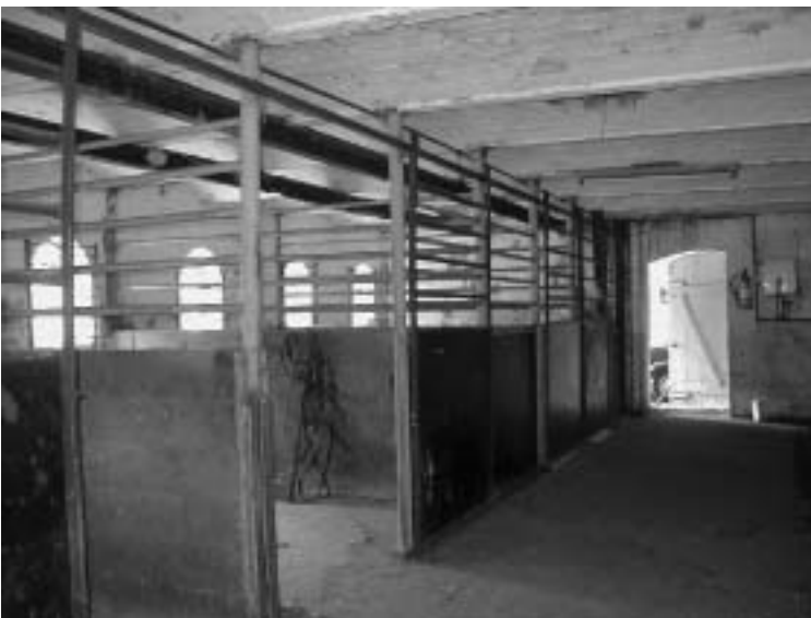
Figure 11.15. Light painted interior reflects more light than a dark interior as shown in this old yet bright whitewashed stable interior.
