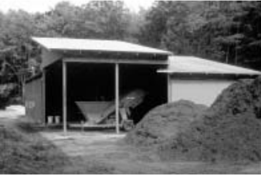
Figure 8.24. Further processing of composted stall waste is often needed prior to sale to provide uniform material. Shredding and sieving are typical processes before being bagged, and even for many bulk sales.
