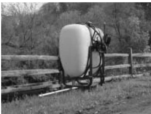
Figure 17.4. A tractor- or pickup-mounted water spray tank: a way to partially automate wetting arena surface materials.
