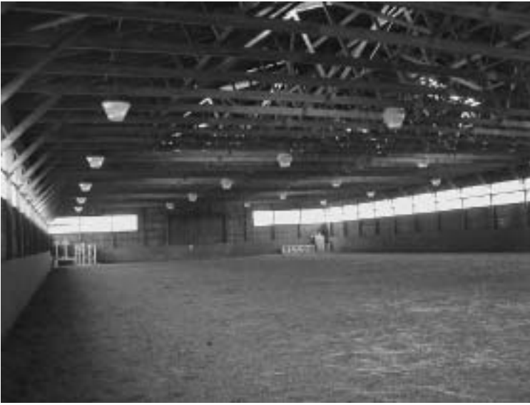
Figure 11.13. Indoor riding arena outfitted with four rows of sealed HID lamps in addition to natural lighting from translucent panels along the top of all walls.
