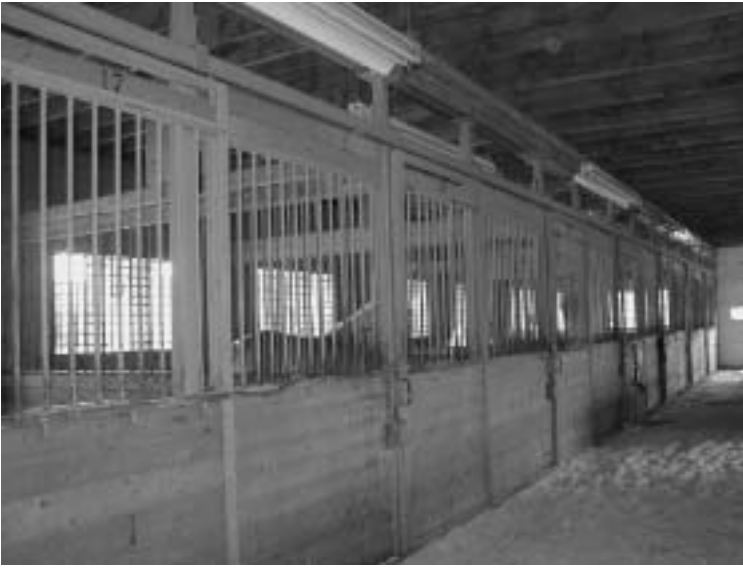
Figure 11.10. Fluorescent fixtures used in aisle and stalls of stable for energy-efficient lighting in cold climate. Locate light fixtures to side of aisle and front of stall to minimize shadows on aisle work and horses, respectively. Fixture location is staggered in aisle and stall to provide more uniform light to both locations.
