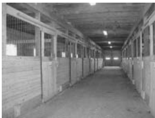
Figure 5.4. Large stable with hay storage in closed loft above a high ceiling. Windows for light and fresh air are provided in each stall. An overhead door provides access to the aisle while sliding doors access each stall.
