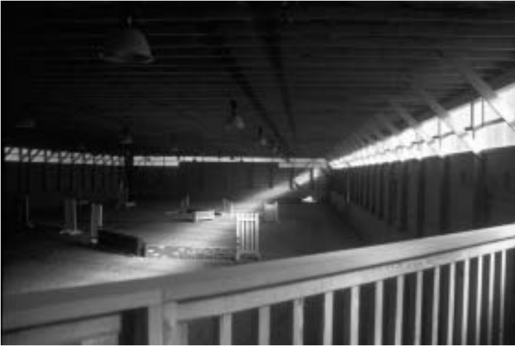
Figure 16.22. Direct light entry through translucent panels results in heat gain, which is often desirable during cold weather, and distinct light and dark floor patterns. (Photo taken from observation deck of Figure 16.21).
