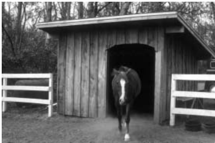
Figure 14.12. Install pasture shelters flush with the fence-line for simple protection of the shelter's exterior building components. A small human-sized gap between fence and shelter wall allows easy access for checking conditions within the shelter.
