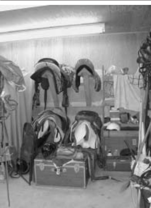
Figure 13.11. Provide a concrete floor in the tack room for easy cleaning and to exclude rodents. Plan room for plenty of shelving and trunks for storing small tack items.
