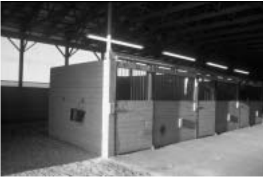
Figure 6.20. Interior view of a racehorse stable that has stalls set up in an island configuration but with central work aisle. Sidewall curtain opening admits plenty of light and fresh air to the facility.
