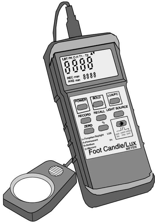
Figure 11.20. Instruments may be used to measure light level at various locations to determine uniformity and overall light level.
