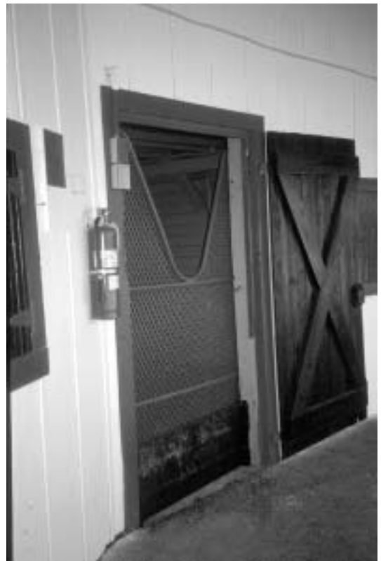
Figure 9.6. Maintain fire extinguishers every 50 feet in large stabling facilities near areas of potential fire such as stalls, hay and bedding storage, and places where equipment or appliances are used. Different types of extinguishers will be needed depending on fire fuel.
