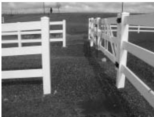
Figure 18.11. Pay special attention to grading for water drainage around heavily used areas such as the arena gate.
