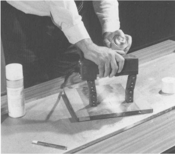
46 Detection of defects using magnetic particle inspection.
