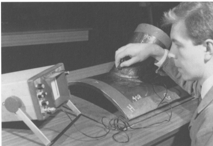
47 Using an ultrasonic probe to detect defects.
