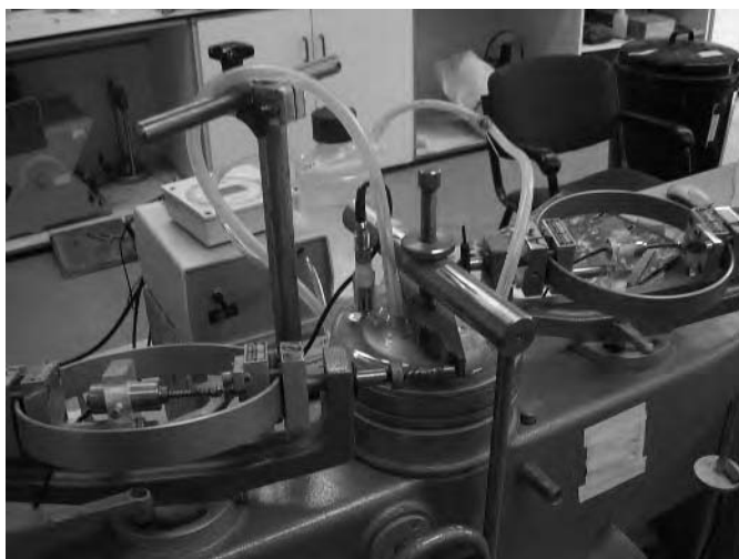
Fig. 1. Adapted general system to control suction on Bromhead ring shear apparatus
