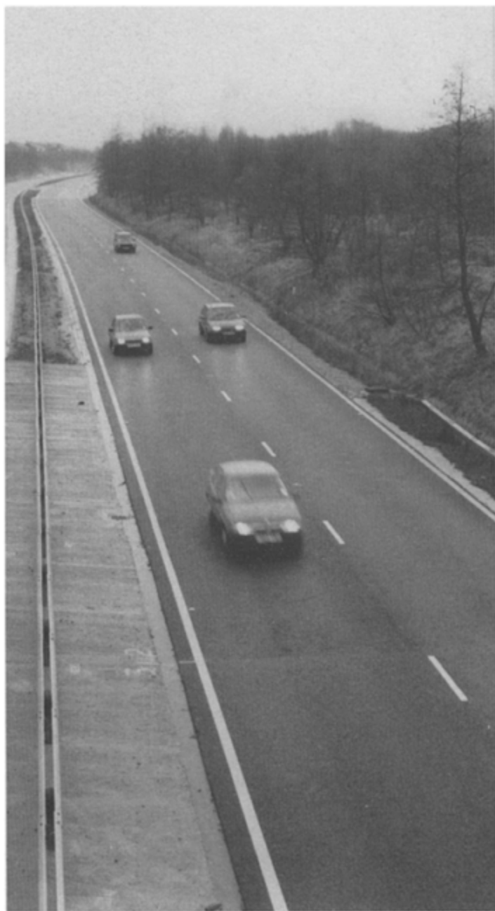
Fig. 7.11 Glare on porous asphalt
