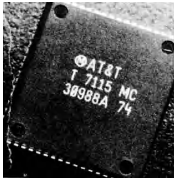
FIGURE 12-1B. No probe targets for gull wing part. These gull wing part leads can be probed from the top, but that is not recommended because the parts tend to shift during the soldering operation.
